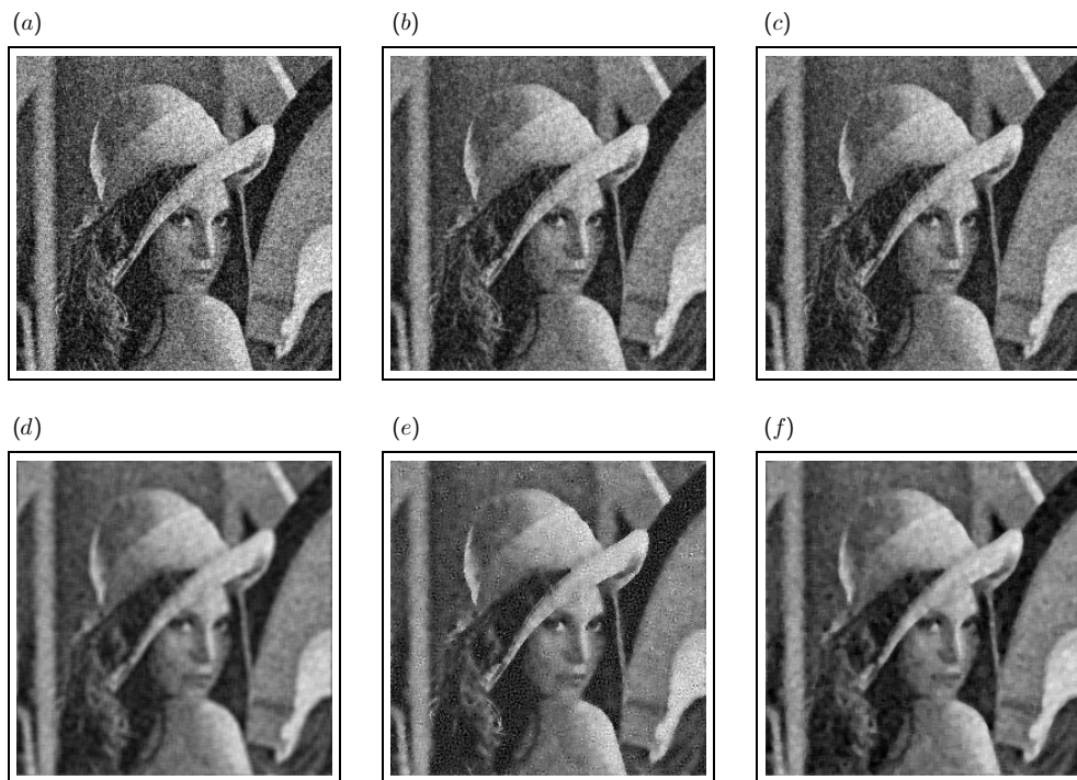
Figure 6. Restored images \hat{f} obtained from the degraded image g given in figure 5(a). (a) Mean-field approximation. (b) Bethe approximation. (c) Exact. (d) Lowpass filter with window size 5 \times 5 . (e) Wiener filter with window size 5 \times 5 . (f) Median filter with window size 5 \times 5 .
